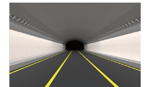
Symmetric against-glare lighting, suitable for angled lighting placement on both sides of the tunnel
