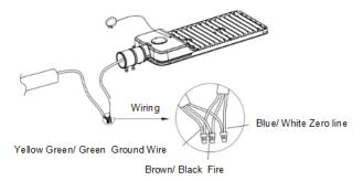
1. Connect the input wire of the fixture with the utility wire of the pole, and connect the corresponding wires as shown in the diagram, and make sure that the color of each connected wire is the same (please refer to the detailed drawing). After connecting, it is necessary to do the corresponding waterproof and anti-pulling treatment.
